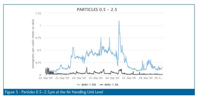
Further, not all particles are the same: larger particles of 10µm stay airborne for a few minutes while smaller particles of 0.3 microns stay airborne for hours. Filter performance is also substantially reduced for smaller particles: A MERV 13 filter is only 40% efficient at 0.3µm while it is 99%+ efficient at 2.5µm! It is not uncommon for 90%+ of all measured particles to be less than 0.5µm.
